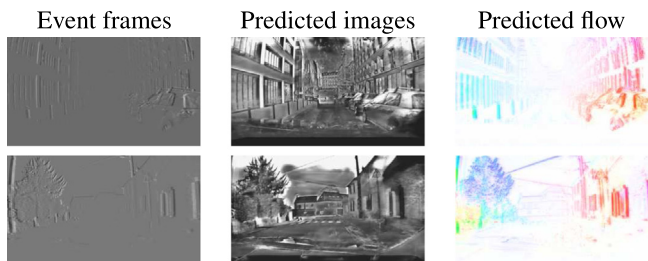
Fig. 7. Reconstruction results obtained from dataset proposed in Perot et al. (2020). The dataset is collected using a 1MP resolution ATIS sensor which acquires only the event sensor data and no intensity frames. We observe that our proposed algorithm is able to generalize well to this new dataset..
